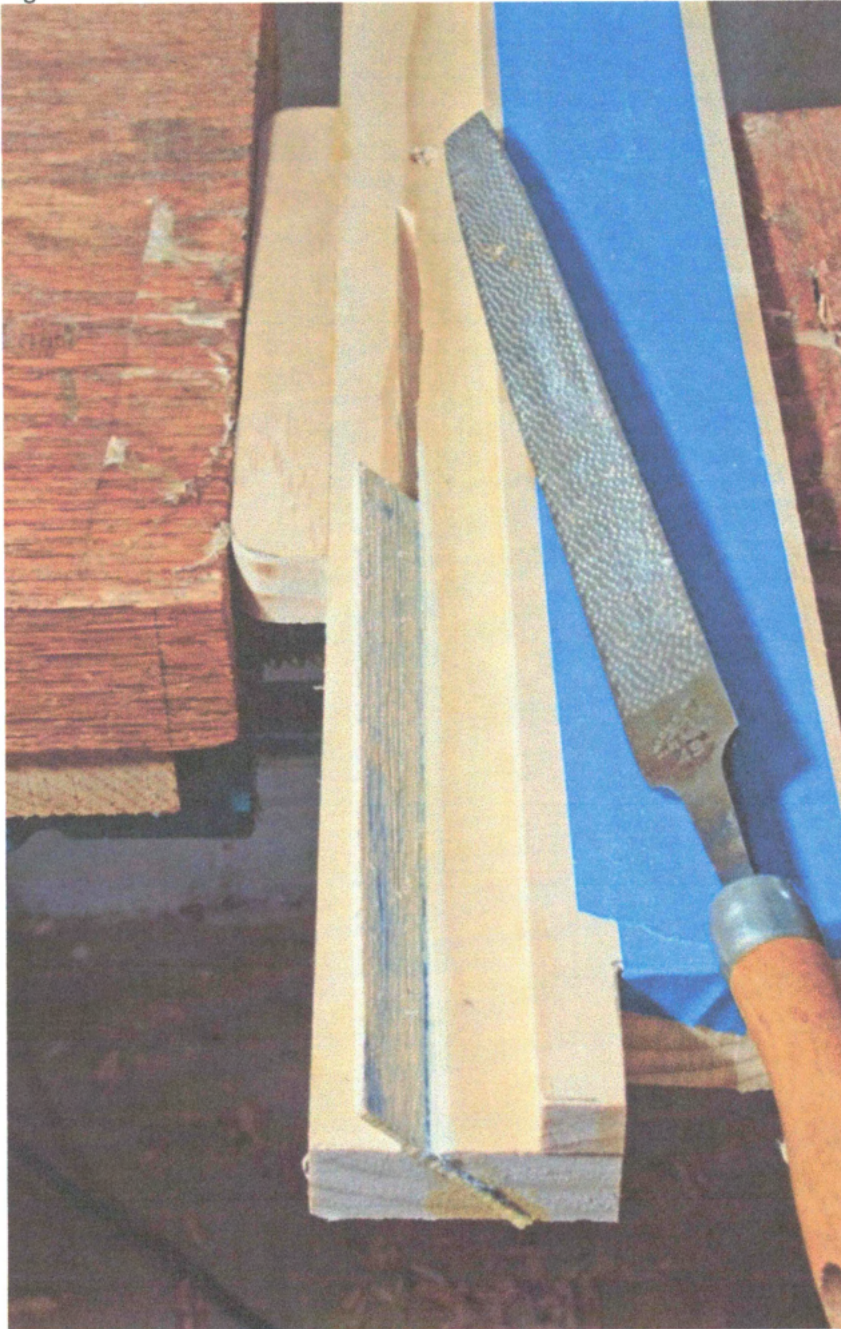
Fig19: Thinning and tapering the splitter.
