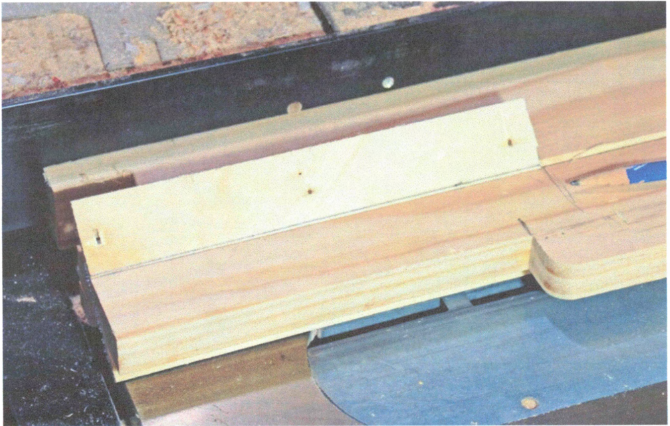
Fig17: Marking the size of the splitter.
