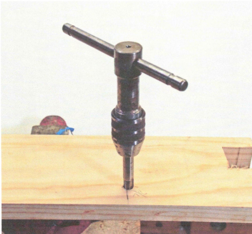
Fig10: Tapping the holes for depth adjusters.
