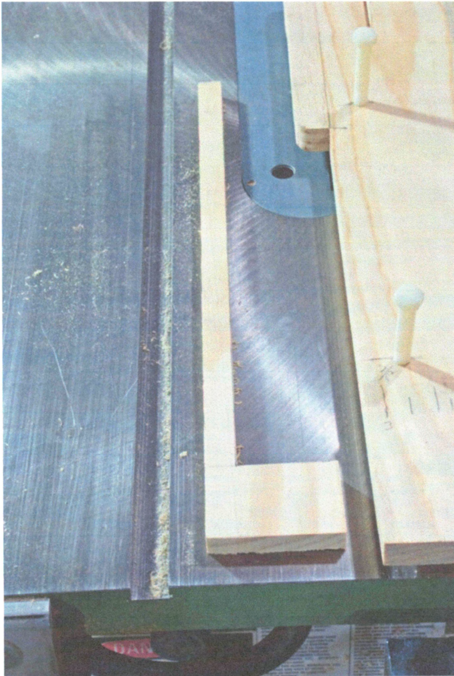
Fig20: The completed half fence.
