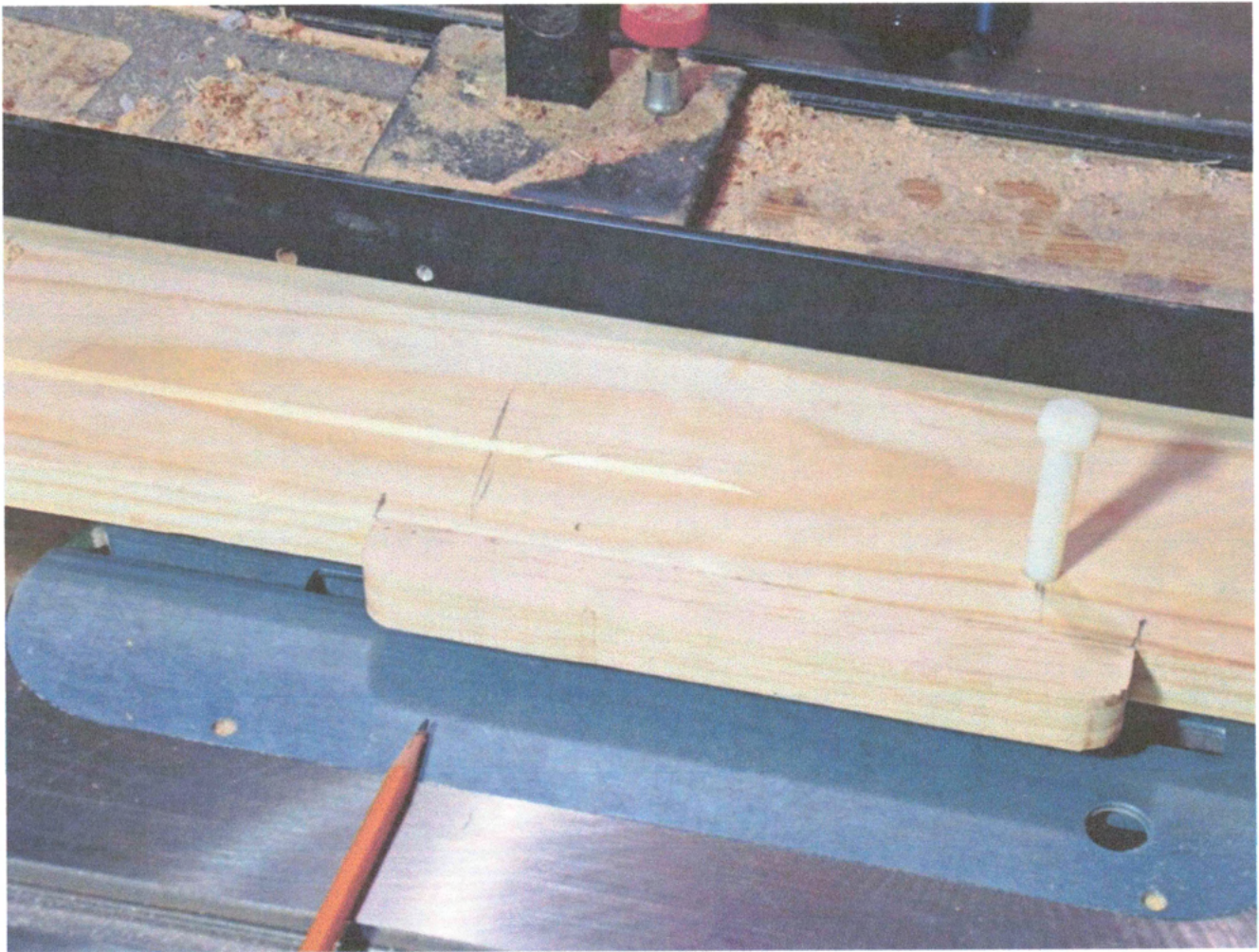
Fig16: Marking for the extent of the splitter.
