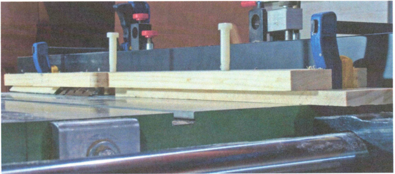
Fig21: The half fence in place.
