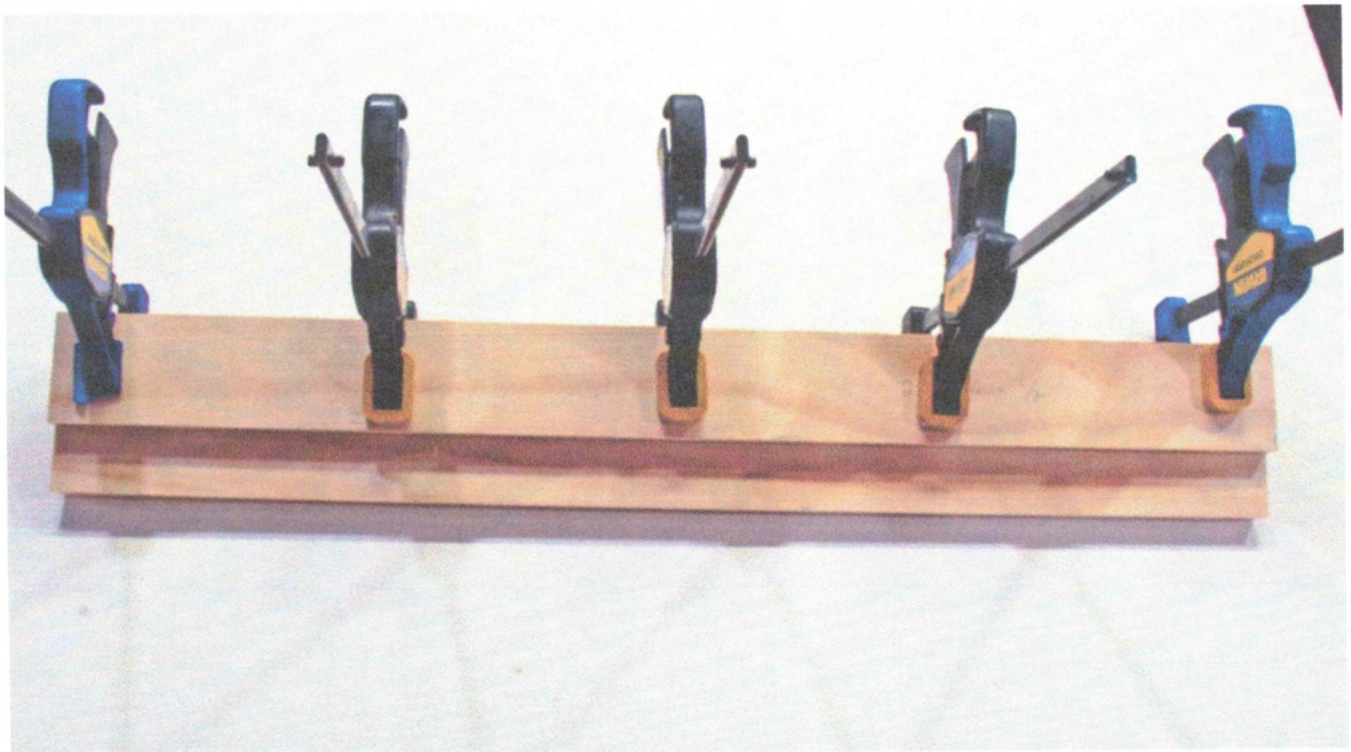
Fig02: Clamping the fence stock while the glue cures.
