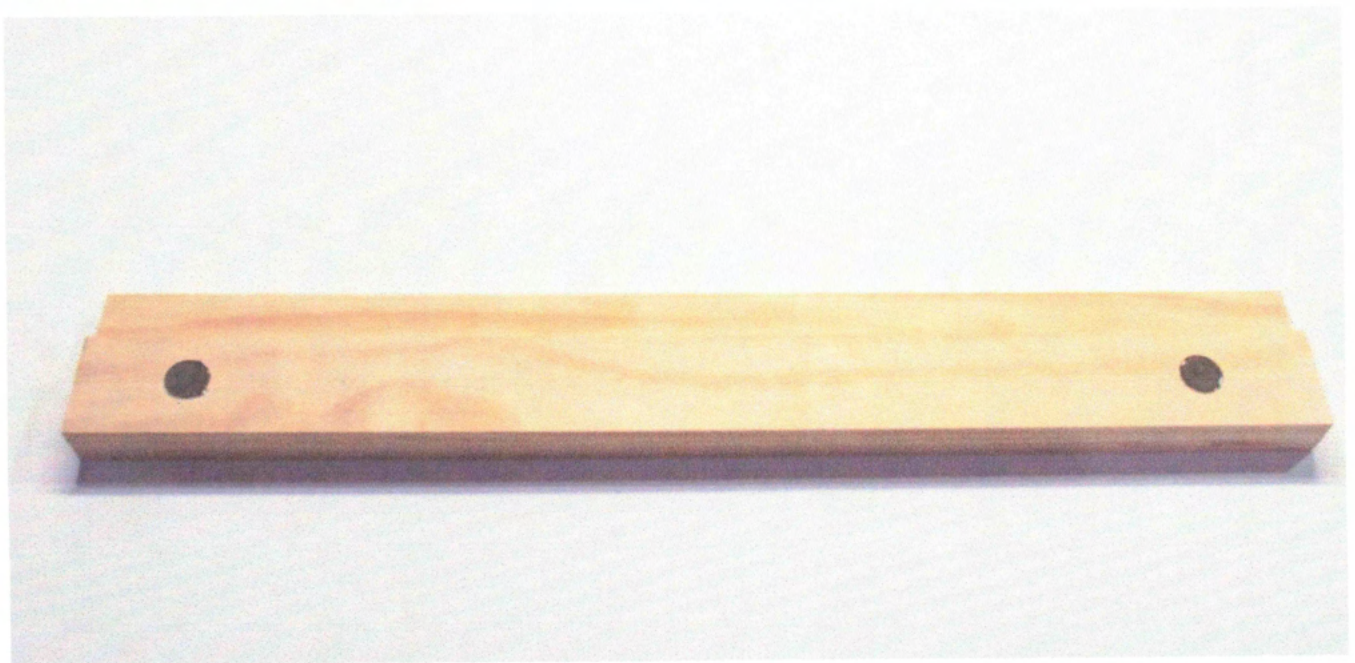
Fig04: Drilling holes for rare earth magnets.
